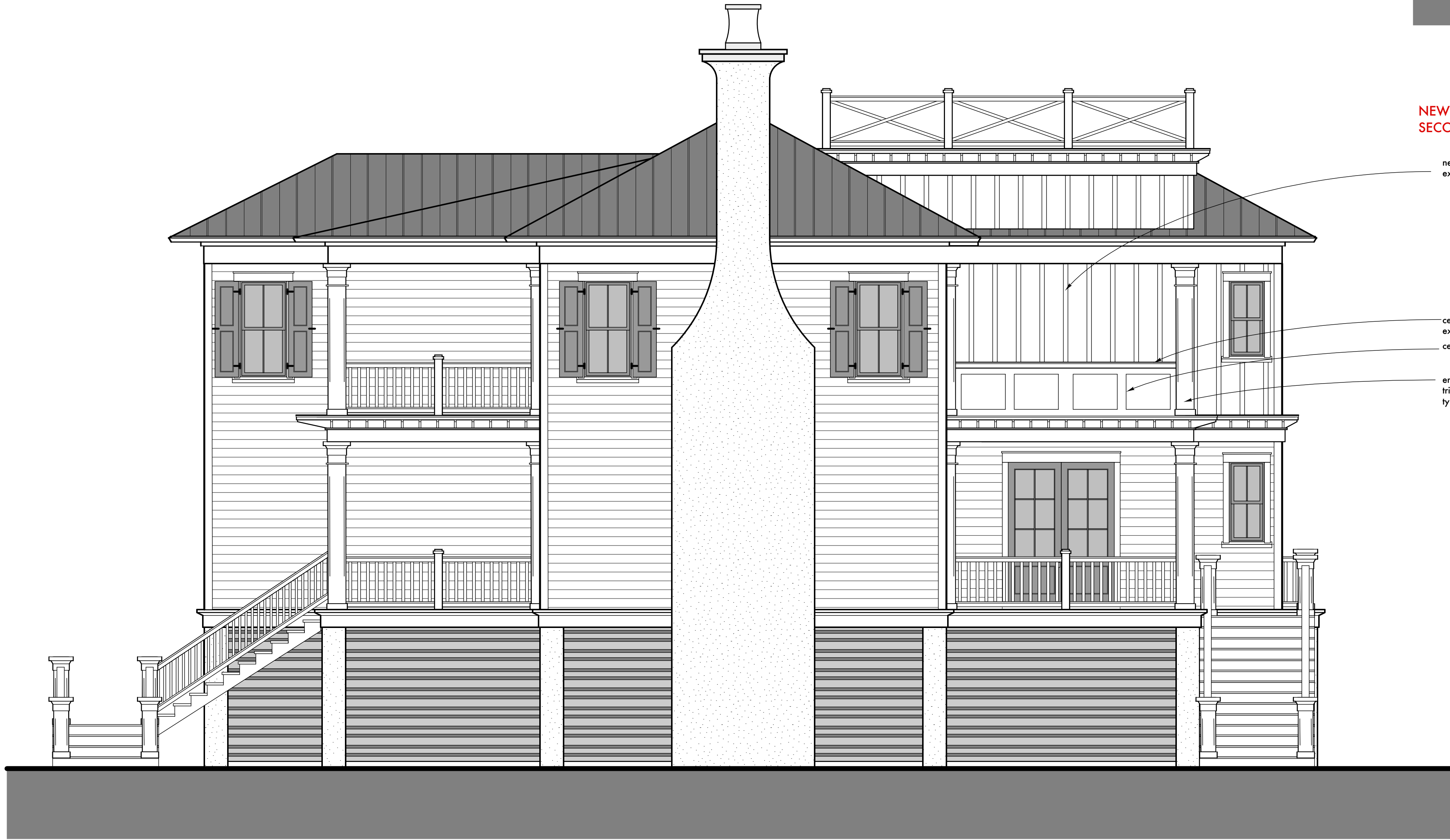
2 Proposed Right Side Elevation with Infill Second Floor Porch Scale: 1/4" = 1'-0"
