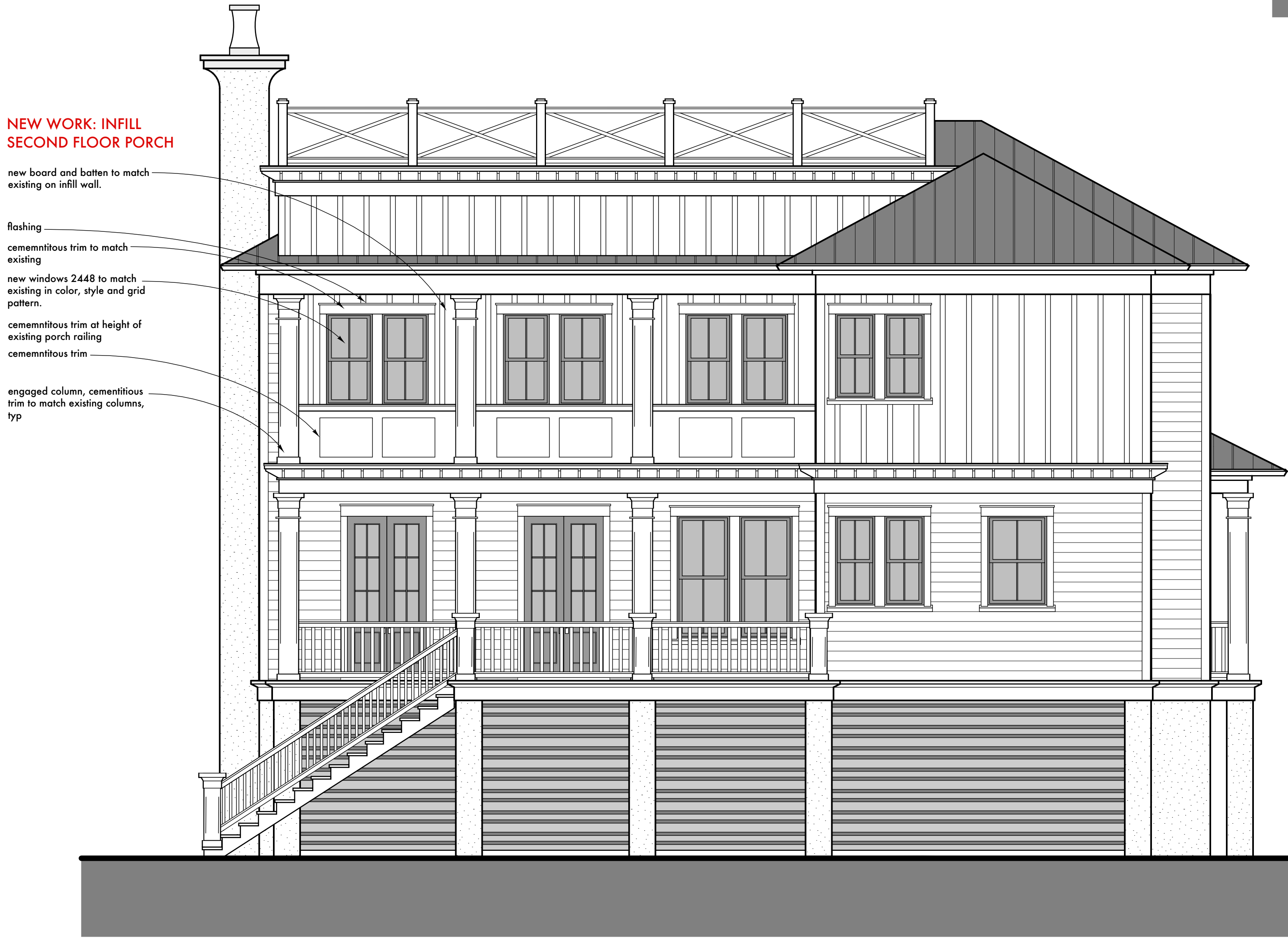
2 Proposed Rear Elevation with Infill Second Floor Porch Scale: 1/4" = 1'-0"
