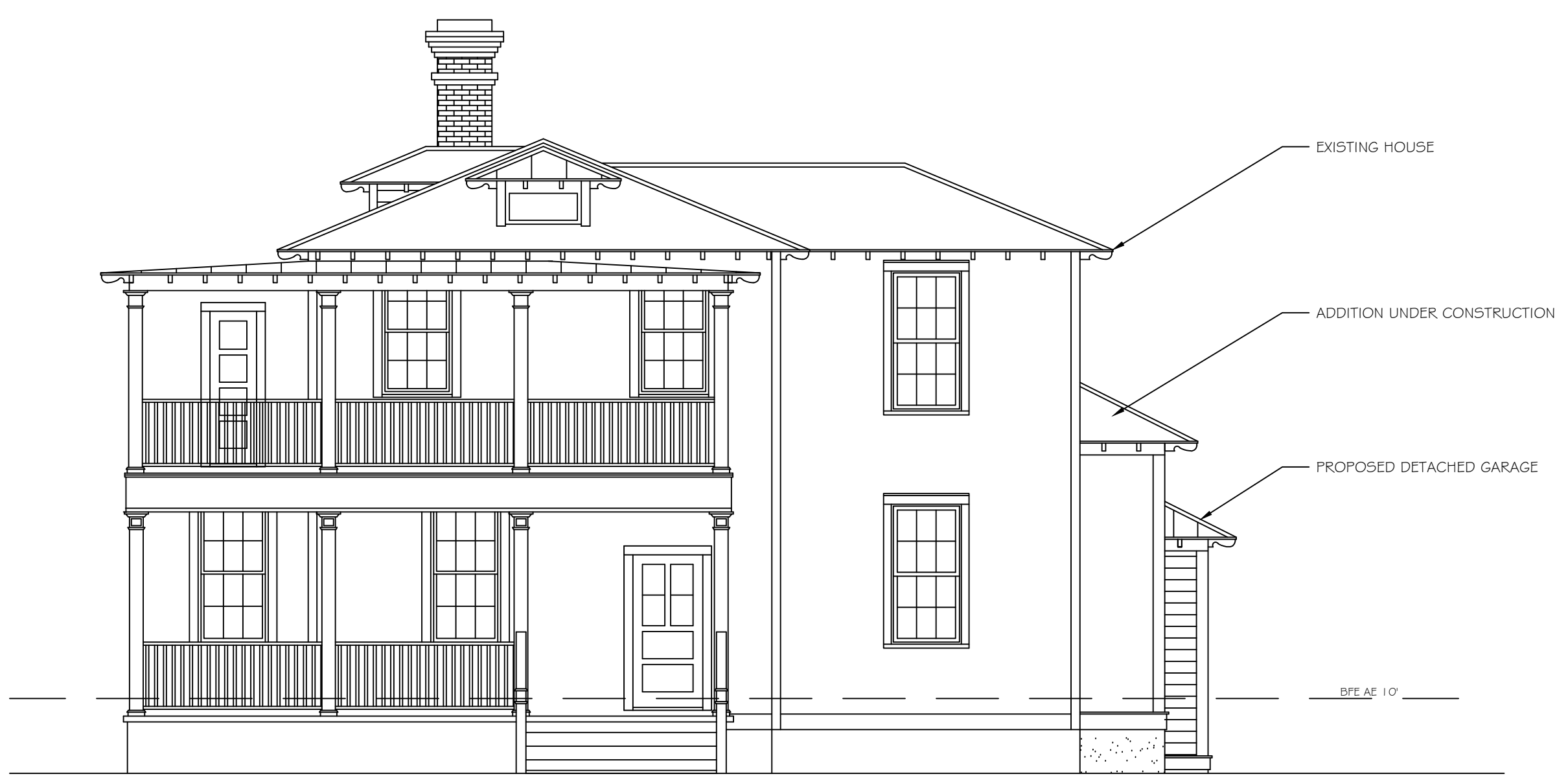
4 PROPOSED FRONT ELEVATION A2
